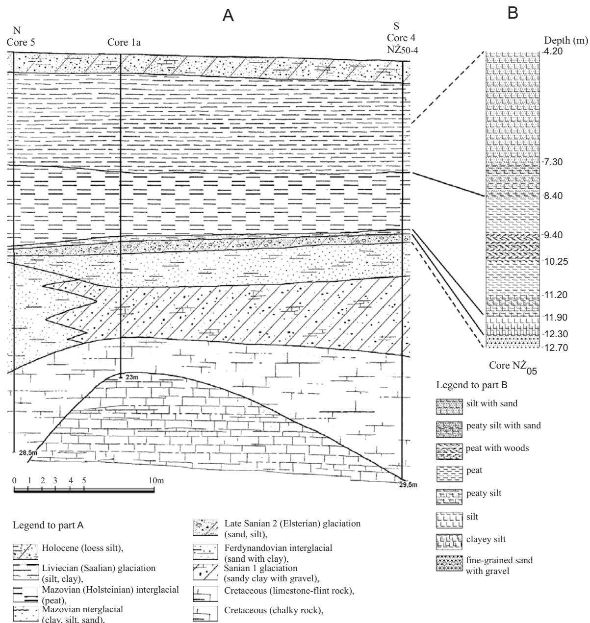
Fig. 2. Geological section of Nowiny Žukowskie: **A** – profile NŽ<sub>50-4</sub> after Rühle (1952); **B** – lithology of NŽ<sub>05</sub> profile
