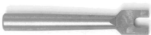
Fig. 31. Manufactured turnbuckle wrench. http://www.rceasy.com/wp-content/uploads/2007/08/79277.JPG , with permission of RCEasy – News on Radio Control Ca.
