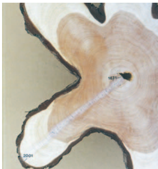
Fig. 3. Section of a 330-year-old, living pine tree, first and last year indicated. Reddish heartwood differs markedly from pale sapwood; a small pocket of decay (white-rot) is seen close to the pith, but otherwise the tree was sound. Finland, Inarin Lappi prov., Inari, August 2001.
